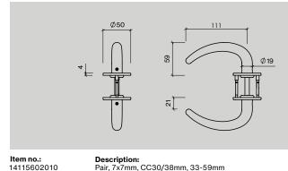
**Description:** Pair, 7x7mm, CC30/38mm, 33-59mm Pair, 8x8mm, CC30/38mm, 33-59mm
