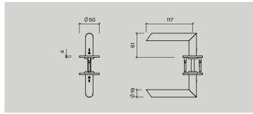
Item no.: 14255602010 14251602010 **Description:** 19FF, oblique, pair, 7x7mm, CC30/38mm, 33-59mm 19FF, oblique, pair, 8x8mm, CC30/38mm, 33-59mm
