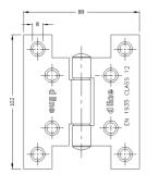
Review of the test observations has shown that the hinges continued to support the door leaves for the full 261 minute duration of the test, notwithstanding the earlier integrity failures of the doorset.
